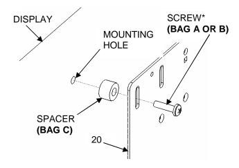
Figure 4. Attaching Interface Bracket to Display
